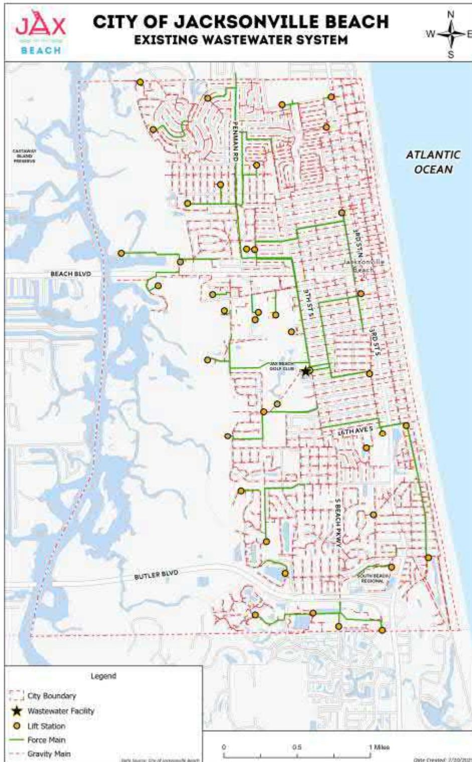
Map PFWM-1: Existing Wastewater System
